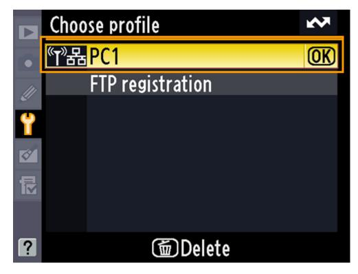
**7–4** Return to the wireless transmitter menu and turn the WT-4 on. The profile name will be highlighted in green when a connection is established.
